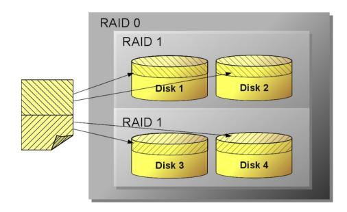
Raid 1+0 / 10: mirrored sets in a striped set the array can sustain multiple drive losses so long as no mirror loses all its drives
